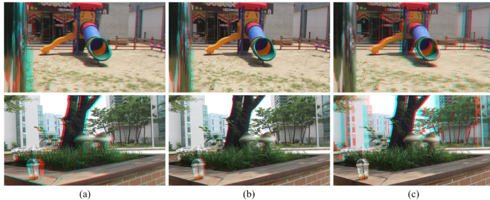
Fig. 7. Results of the two-stage optimization: (a) the anaglyph image of Scheme-A, (b) the anaglyph image of Scheme-B, and (c) the anaglyph image of our approach.
